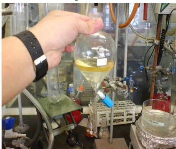
Fig. 1 c. Laboratory-scale liquid-liquid extraction. Photograph of a separatory funnel in a laboratory scale extraction of 2 immiscible liquids: liquids are a diethyl ether upper phase, and a lower aqueous phase.
