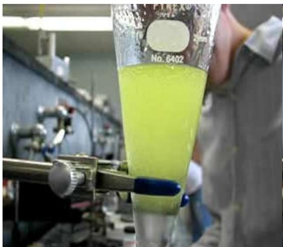
Fig. 1 a. Process of transfer of a dissolved substance from one phase to another phase, which are immiscible or restrictedly miscible, is called liquid-liquid –partition or partition between two phases of liquids.
